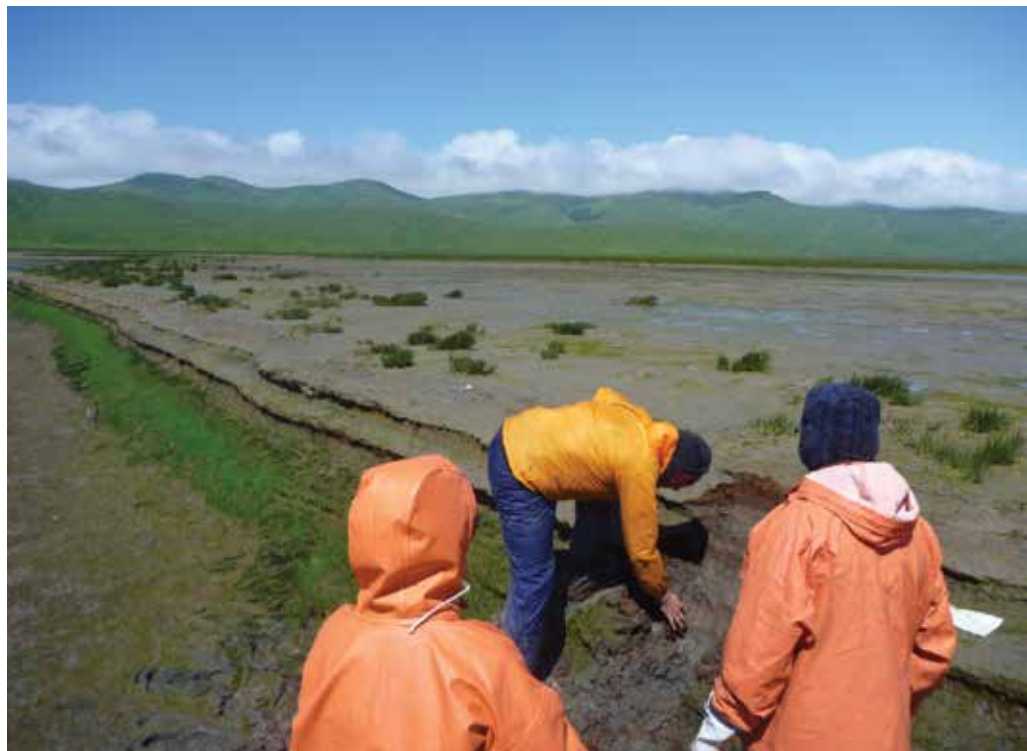
Researchers (left to right) Andrew Kemp, Peter Haeussler, and Alan Nelson examine salt marsh beds in a tidal outcrop on Sitkinak Island, Alaska. These beds provide evidence of earthquake-induced changes in land level, including coastal uplift during the 1788 earthquake. Credit: USGS
